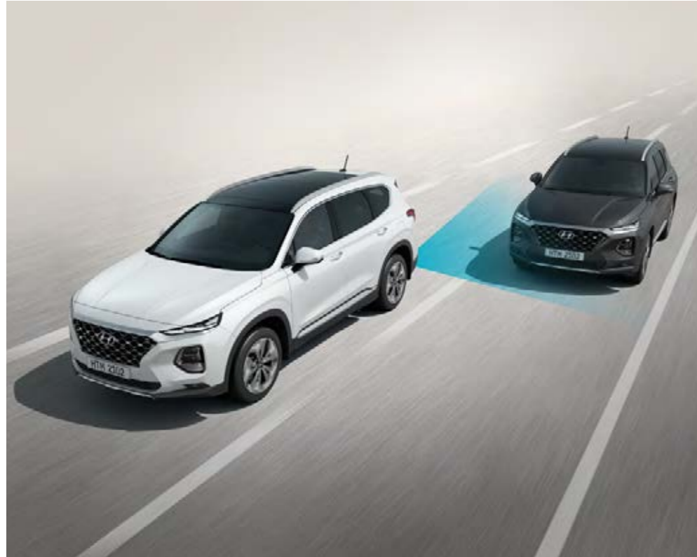
Blind-Spot Collision Warning (BCW) Radar sensors in the rear bumper are used to warn the driver of approaching vehicles in the blind spot area.
