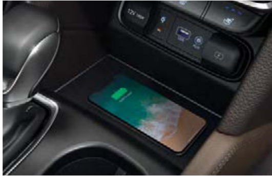
Wireless Smartphone Charging System
