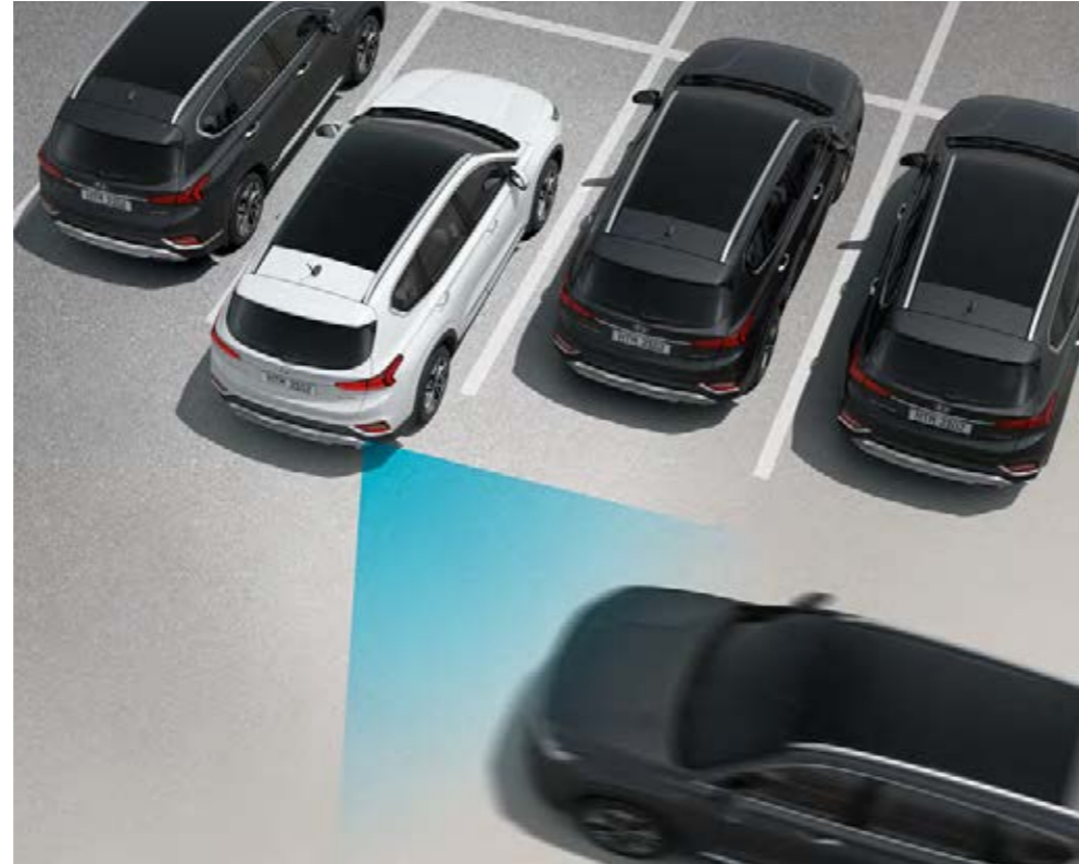
Rear Cross-Traffic Collision Warning (RCCW) Radar sensors in the rear bumper alert the driver about cross traffic approaching from left and right side of the vehicle during reverse maneuvers.
